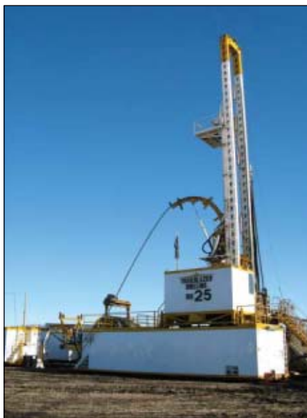
Calgary's Savanna Energy Services Corp. has 46 hybrid drilling rigs in its fleet, capable of running coiled tubing or conventional jointed pipe with top drives and automated pipe-handling equipment (Fig. 2; photo from Savanna Energy).
